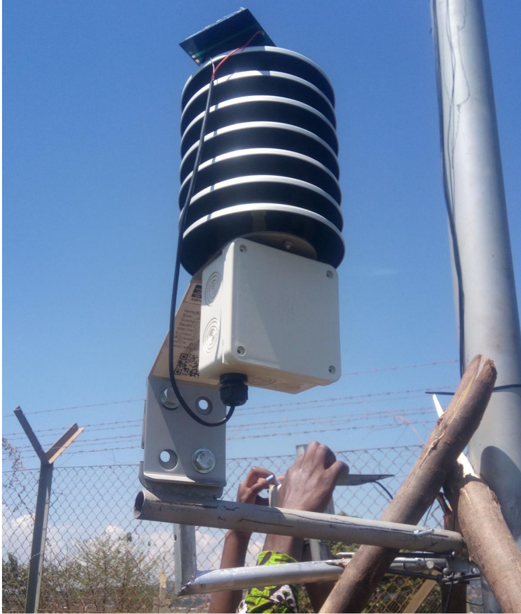
Figure 7. Protrusions for attaching sensors, approximately 2m from the ground and showing how the 2m node is attached.
