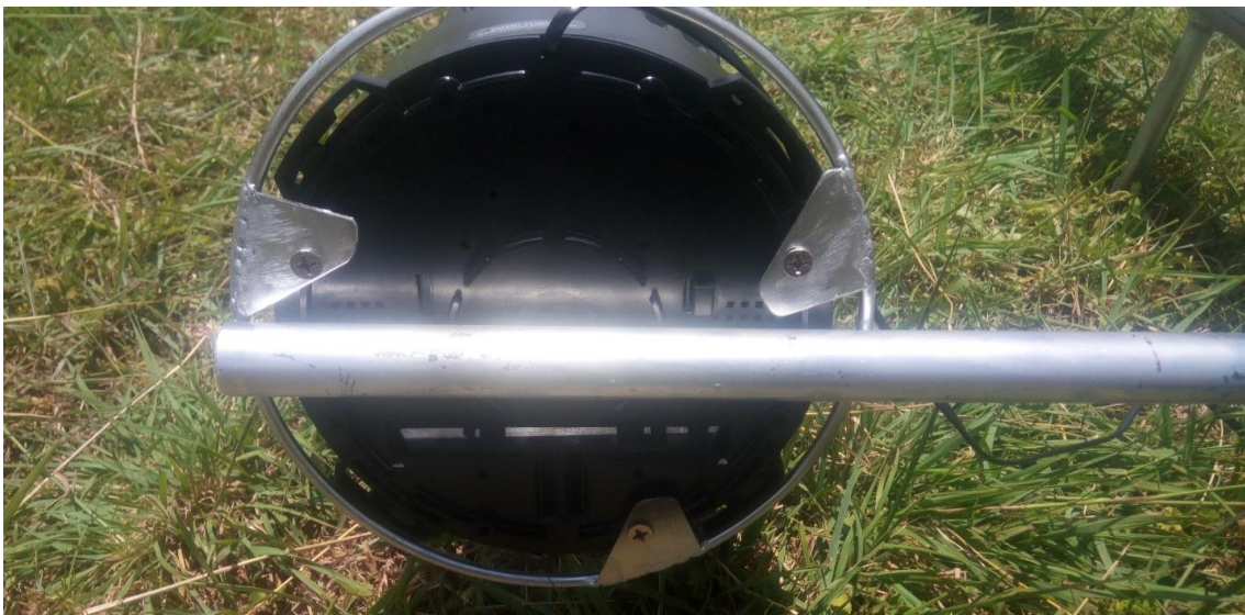
Figure 5. Rain gauge fixed to its base. The hollow pipe has a diameter of 25mm to enable it enter into another pipe, which is attached to the stand
