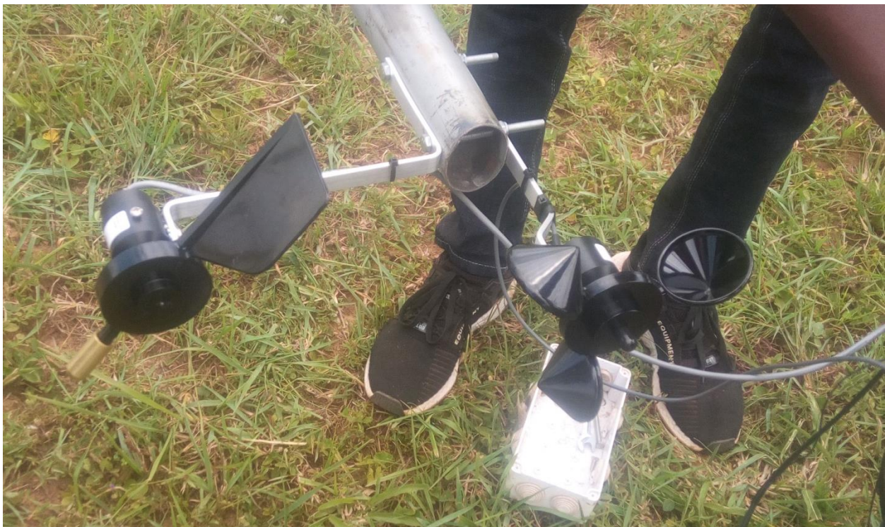
Figure 9. Attaching the wind sensors to the top metallic pipe
