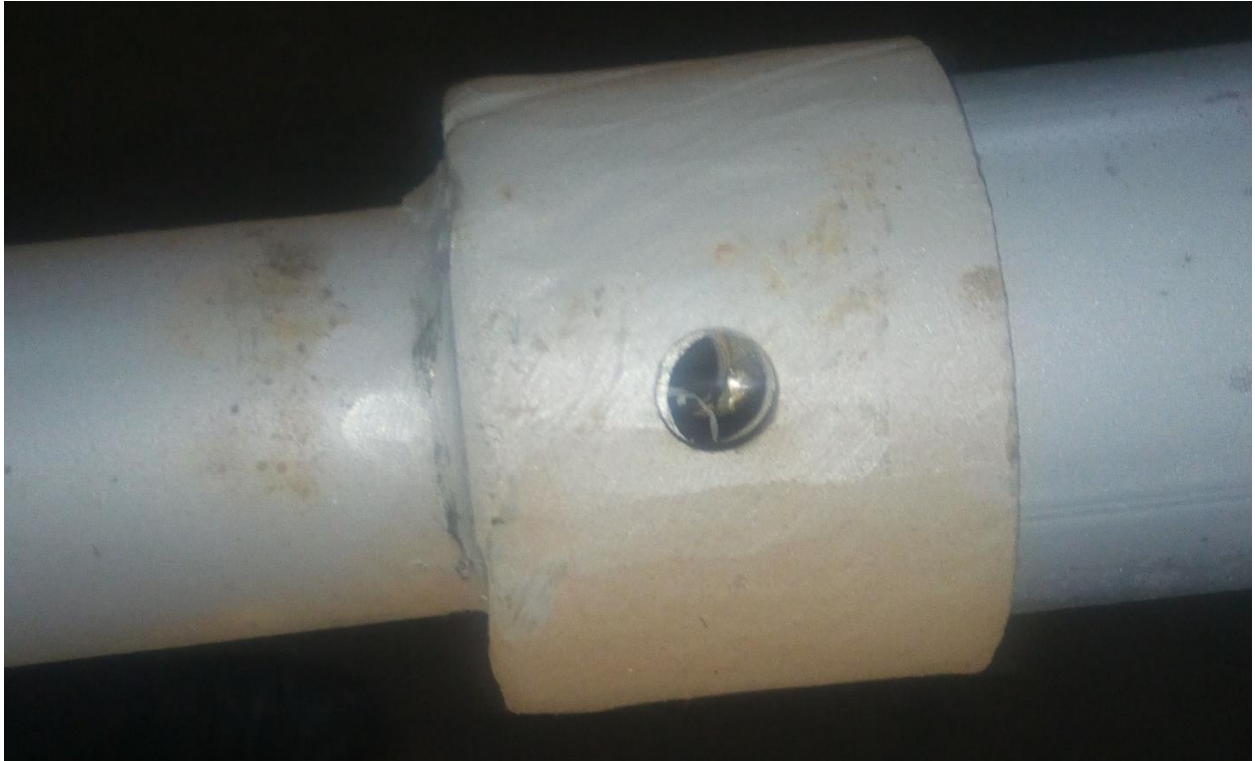
Figure 2. Joint attached to the smaller pipe, to make it fit in the bigger diameter lower pipe. The hole is for tightening the pipes during deployment
